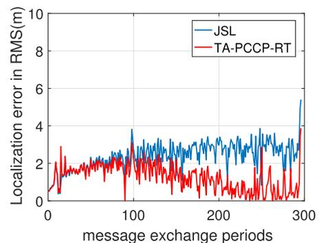
**FIGURE 13.** Localization error comparison between JSL and PCCP in the deep sea experiment.
