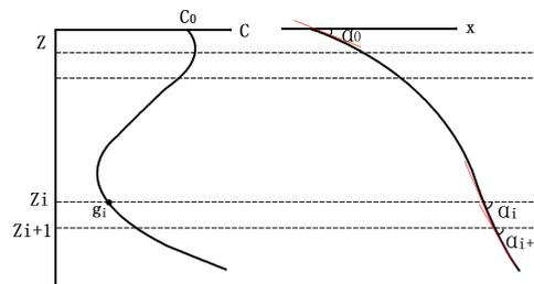
**FIGURE 3.** Ray tracing algorithm.
