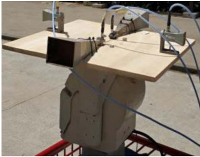
Fig. 2. High-gain horn antenna equipped with the digital turntable.
