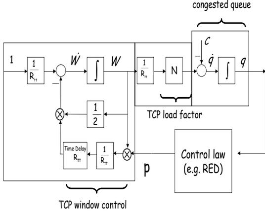
Fig. 2. Block Diagram of AIMD/RED Network
