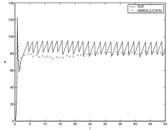
Fig. 14. TCP and AIMD(0.2, 0.875) window trace
