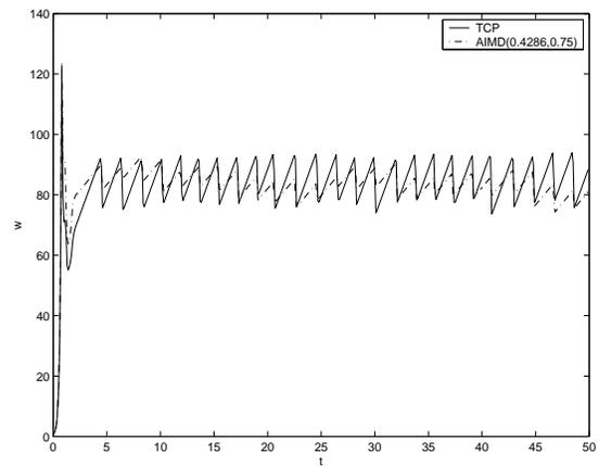
Fig. 15. TCP and AIMD(0.4286, 0.75) window trace
