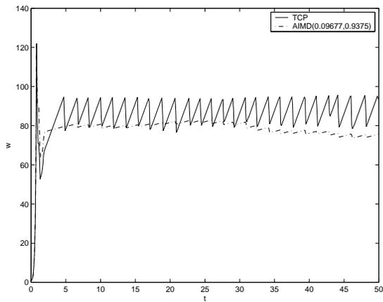
Fig. 13. TCP and AIMD(0.09677, 0.9375) window trace
