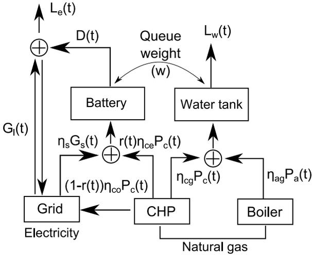
Fig. 1. CHP system uses natural gas.
