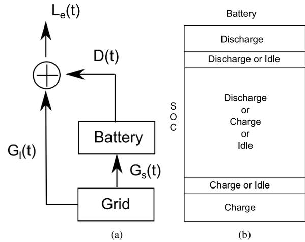
Fig. 2. Simplified battery system. (a) System model. (b) Battery model.
