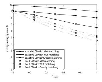
Fig. 9. Average energy gain vs. normalized velocity.
