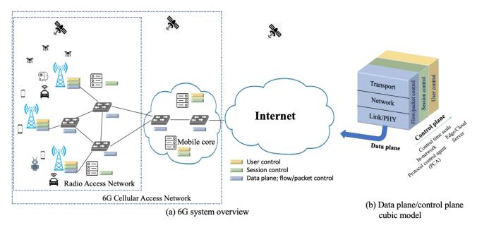
Fig. 3. 6G system overview and data/control-plane protocol model.
