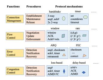
Fig. 4. Decomposition of the transport layer control functions.
