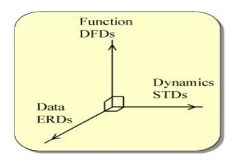
Note: -DFD: Data Flow Diagram -ERD: Entity-Relation Diagram -STD: State Transition Diagram
