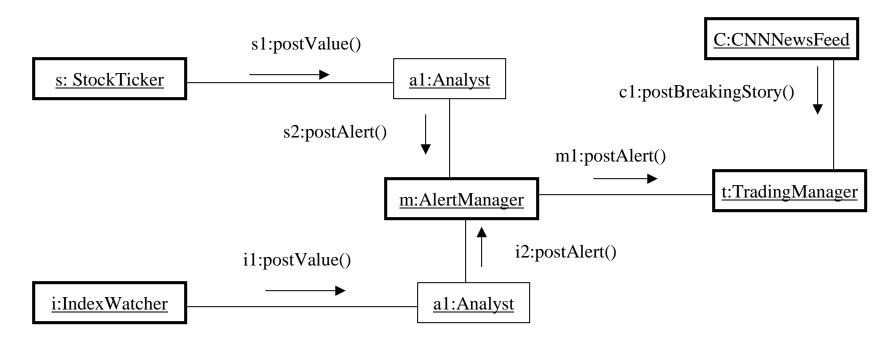
•Interaction diagrams such as these are useful in helping you to visualize where two flows of control might cross paths, and therefore where special attention must be paid to communication and synchronization problems.
