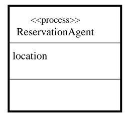
An *Active Object* is an object that owns a process or thread and can initiate control activity.
