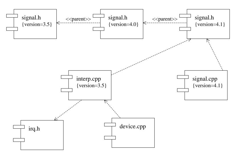
•Based on this component diagram, it is easy to trace the impact of changes. For example, changing the source code file signal.h will require recompilation of three other files: signal.cpp, interp.cpp, and transitively device.cpp. However, file irq.h is not affected.
