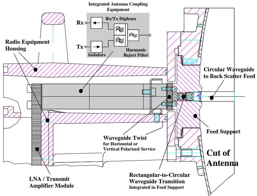
Figure 1. Antenna feed system for a short haul radio featuring an integrated antenna/transceiver solution (Marconi)
