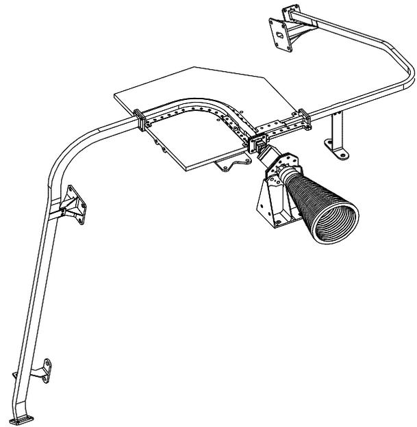
Figure 2. Koreasat-3 Ka-band antenna feed.
