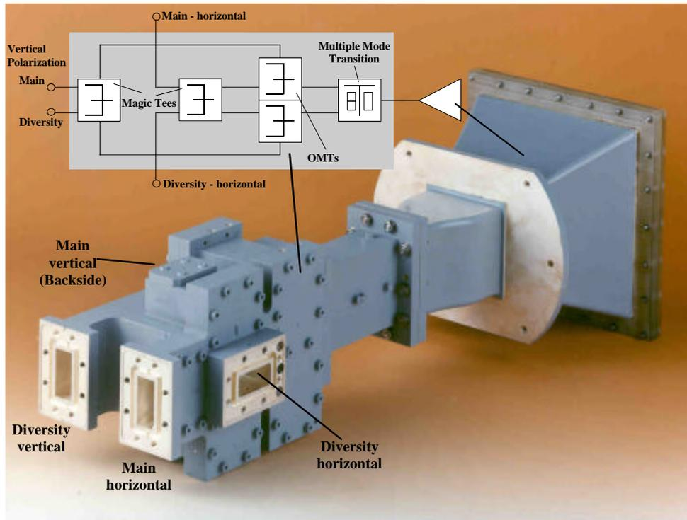
Figure 3. 6GHz dual polarized integrated angle diversity feed system, based on multiple mode excitation for the generation of independent horizontal and vertical main and diversity beams (Marconi)
