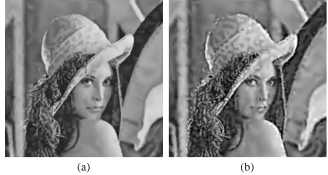
Fig. 5. Lossy reconstructed images obtained at about 50:1 compression with the (a) MGH (26.91 dB) and (b) MGH-CT (23.76 dB) methods.
