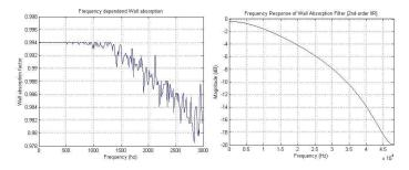
Fig. 4. 2nd-order IIR approximation of wall filter
