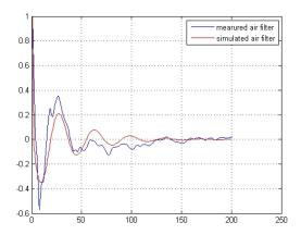
Fig. 3. 2nd-order IIR approximation of air filter
