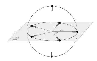
Fig. 1. Microphone Array
