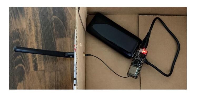
Coach's device prototype developed using Raspberry Pi and RAK 2245 LoRaWAN gateway.
