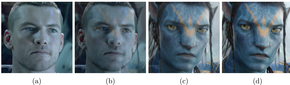
Figure 1.1: An example of image morphing. (a) The source image. (d) The target image. (b) and (c) Intermediate frames generated by applying an image-morphing technique.
