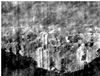
Magnitude Spectrum from Image A and Phase Spectrum from Image B
