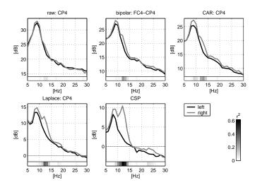
Fig. 4. Spectra of left vs. right hand motor imagery. All plots are calculated from the same dataset but using different spatial filters. The discrimination between the two conditions is quantified by the  $r^2$ -value. CAR stands for common average reference.
