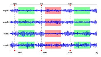
Fig. 5. Effect of spatial CSP filtering. CSP analysis was performed to obtain 4 spatial filters that discriminate left from right hand motor imagery. The graph shows continuous band-pass filtered EEG after applying the CSP filters. The resulting signals in filters CSP:L1 and CSP:L2 have larger variance during right hand imagery (segments shaded in green) while signals in filters CSP:R1 and CSP:R2 have larger variance during left hand imagery (segment shaded red).
