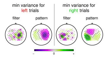
Fig. 7. Example of CSP analysis. The patterns  $(a_j)$  illustrate how the presumed sources project to the scalp. They can be used to verify neurophysiological plausibility. The filters  $(w_j)$  are used to project the original signals. Here they resemble the patterns but their intricate weighting is essential to obtain signals that are optimally discriminative with respect to variance. See Sec. III-B for the definition of the terms *filter* and *pattern*.
