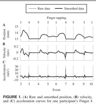
motion during two tapping cycles of the 3-1-4-5 sequence. Vertical lines mark the arrival time of each tap.
