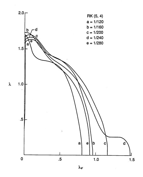
FIGURE 3. Comparison of optimized RK[5,4] schemes with conventional RK[3,3] and RK[4,4] schemes.
