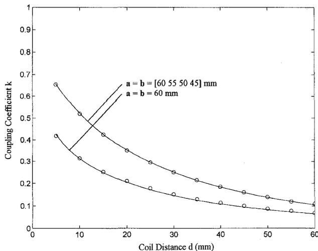
Fig. 4. Coupling coefficient as a function of the coil distance for coil configurations  $a = b = [60 \ 55 \ 50 \ 45]$  mm (upper curve) and  $a = b = 60$  mm (lower curve). Solid curves are the computed results, circles indicate experimental data. The wire radius is  $R = 0.2$  mm.
