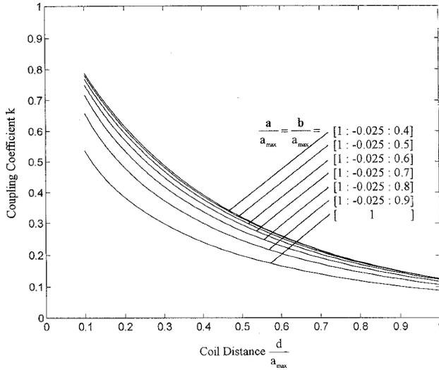
Fig. 2. Coupling coefficient  $k$  as a function of spacing for various coil configurations. Primary and secondary coils are assumed to be identical. The normalized wire radius is  $\frac{R}{a_{\max}} = 12.5 \times 10^{-3}$ .
