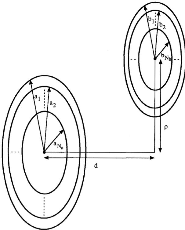
Fig. 1. Geometric arrangement and notation for primary and secondary coils composed of circular concentric loops.
