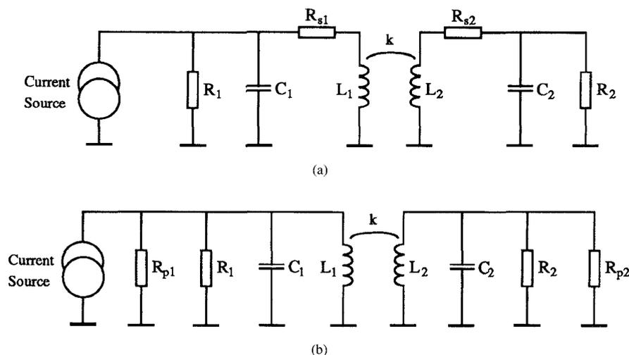
Fig. 6. (a) Circuit diagram of an inductive RF-link and (b) approximated circuit.
