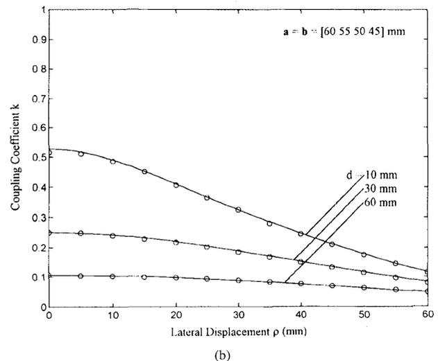
Fig. 5. Coupling coefficient as a function of the lateral displacement for coil separations  $d = 10, 30,$  and  $60$  mm. Solid curves are the theoretical results, circles indicate experimental data. The wire radius is  $R = 0.2$  mm: (a) Single-turn coils  $a = b = 60$  mm and (b) "Distributed" coils  $a = b = [60 \ 55 \ 50 \ 45]$  mm.
