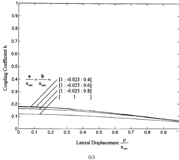
Fig. 3. (Continued). Coupling coefficient as a function of the normalized lateral displacement  $\frac{\rho}{a_{\max}}$  for identical primary and secondary coils. In each plot, four coil configurations  $\frac{a}{a_{\max}} = \frac{b}{a_{\max}} = [1, [1: -0.025: 0.8], [1: -0.025: 0.6],$  and  $[1: -0.025: 0.4]$ , with increment  $\Delta = 2R$  are considered. The normalized wire radius is  $\frac{R}{a_{\max}} = 12.5 \times 10^{-3}$ . The coil distance is: (c)  $\frac{d}{a_{\max}} = 0.8$ .
