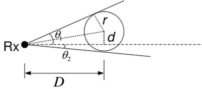
Figure 4: Computation of LOS Blocking Angular Range
