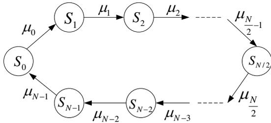
Figure 7: Packet-level Model of Time-varying UWB Channel
