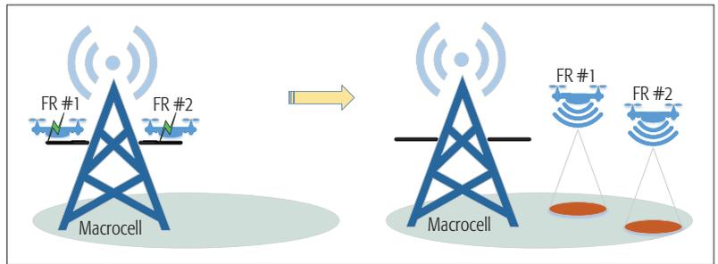
FIGURE 1. The basic concept of the UABS.
