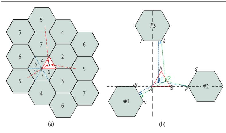
FIGURE 3. An example of the frequency allocation and the topology of interference.
