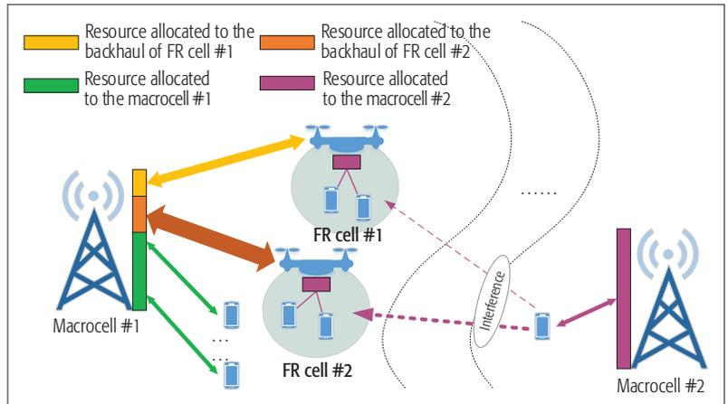
FIGURE 2. Frequency allocation for the FR cells and corresponding interference.
