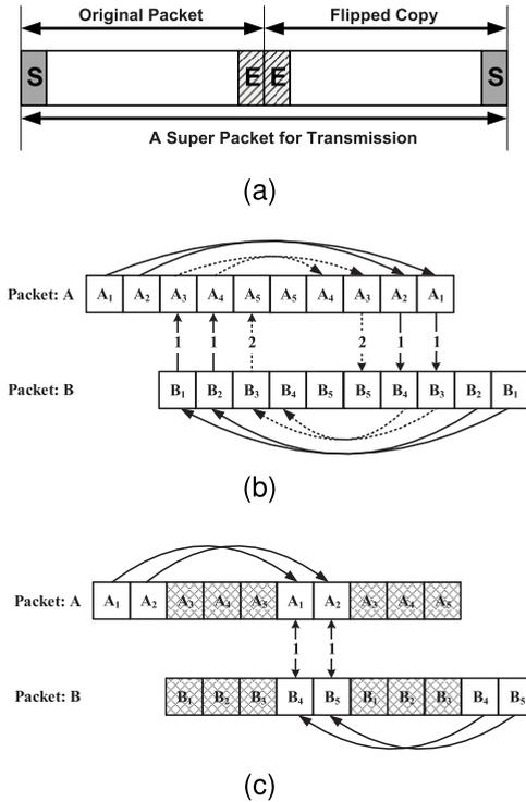
**FIGURE 2.** Collision Resolution in AFDA (The shadowed chunks in Fig. 2c represent the overlapped parts of packets, which cannot be decoded.) (a) super packet. (b) Zigzag decoding in AFDA. (c) Failed decoding without packet flipping.
