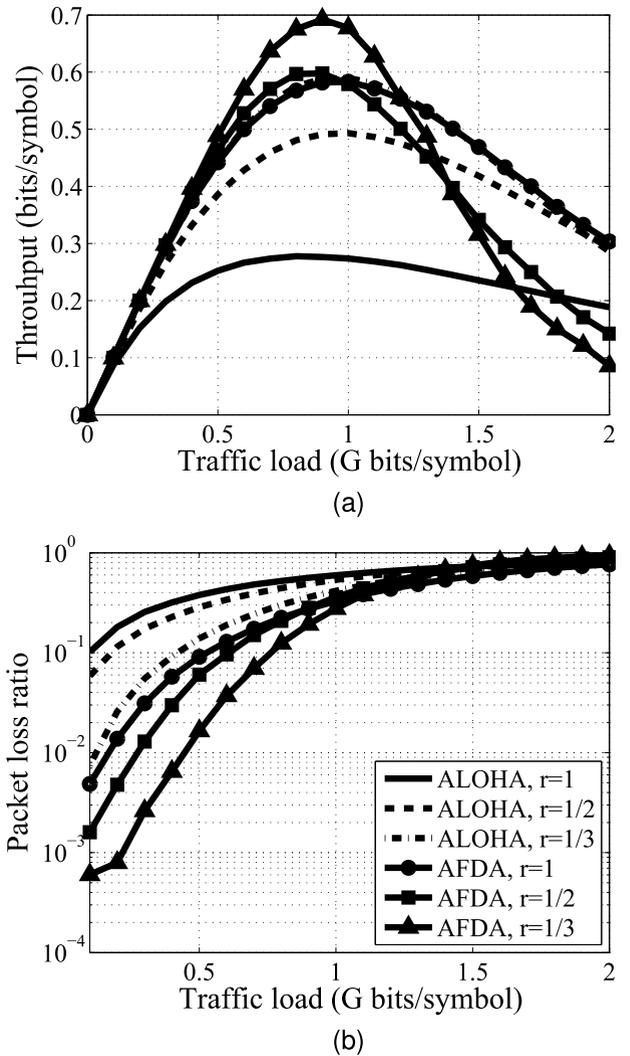
**FIGURE 6.** AFDA performance with variable packet length, simulation results (The legends in the two sub-figures are the same. To avoid the overlap between the curves and their legends, legends are only marked in sub-figure b.) (a) Throughputs. (b) Packet loss ratios.
