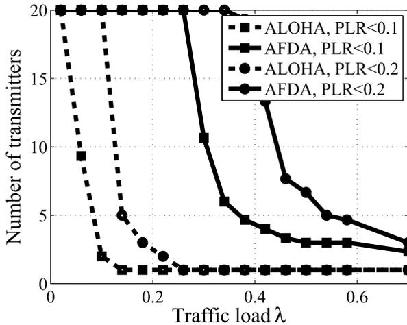
FIGURE 7. Maximum admissible number of transmitters, simulation results.
