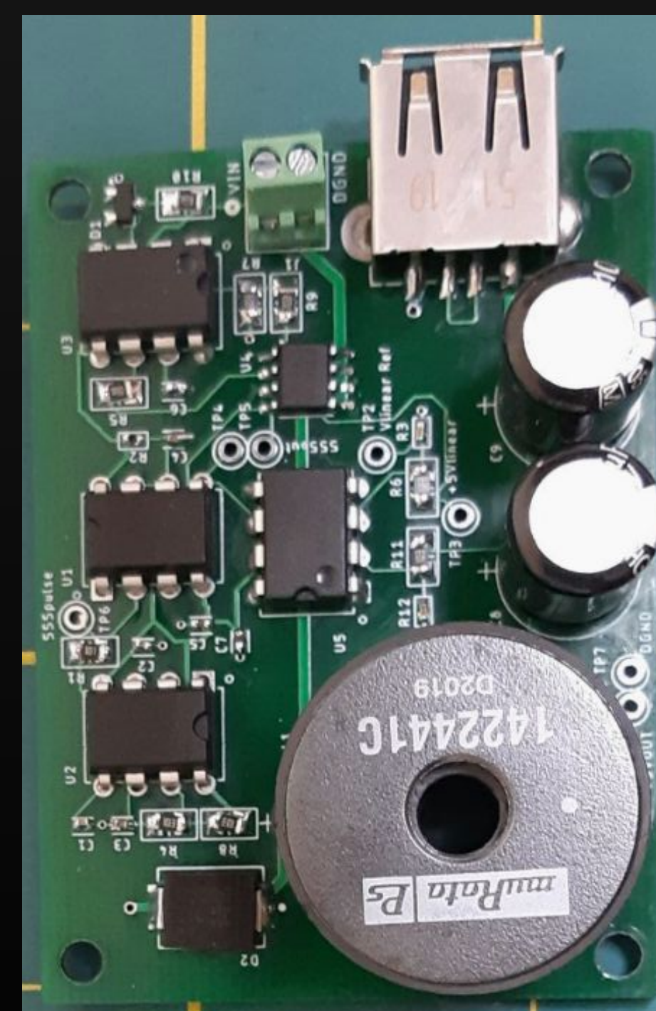
NE555 Timer Switching Regulator
