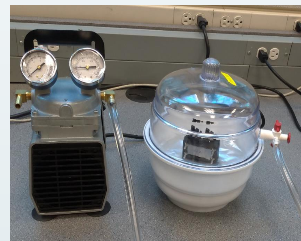
Silicone was degassed before and after injection into the molds
