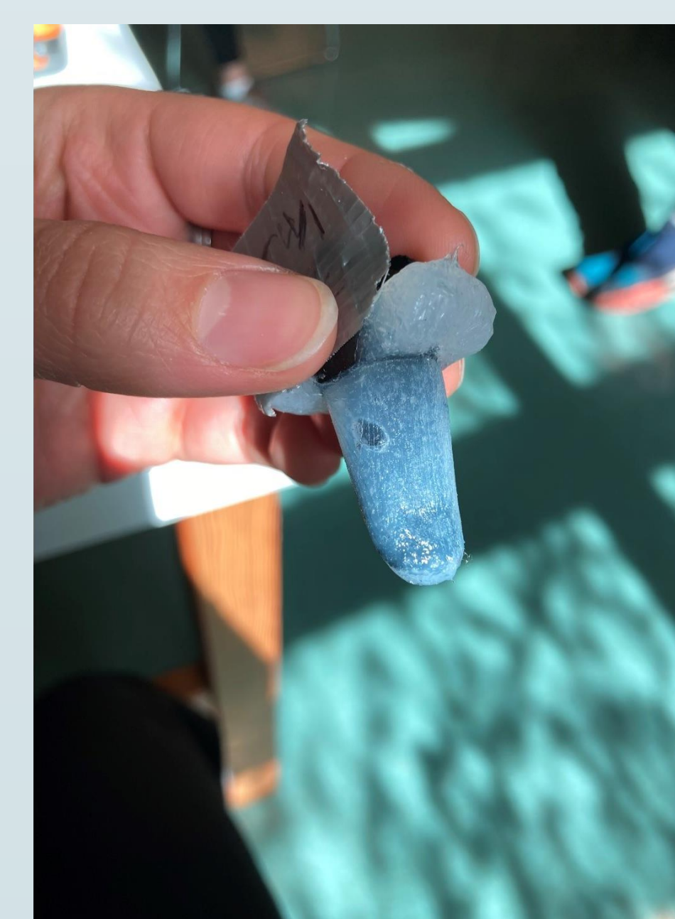
Finger Produced from Mold 1 with Reduced Viscosity and 2x Degassing
