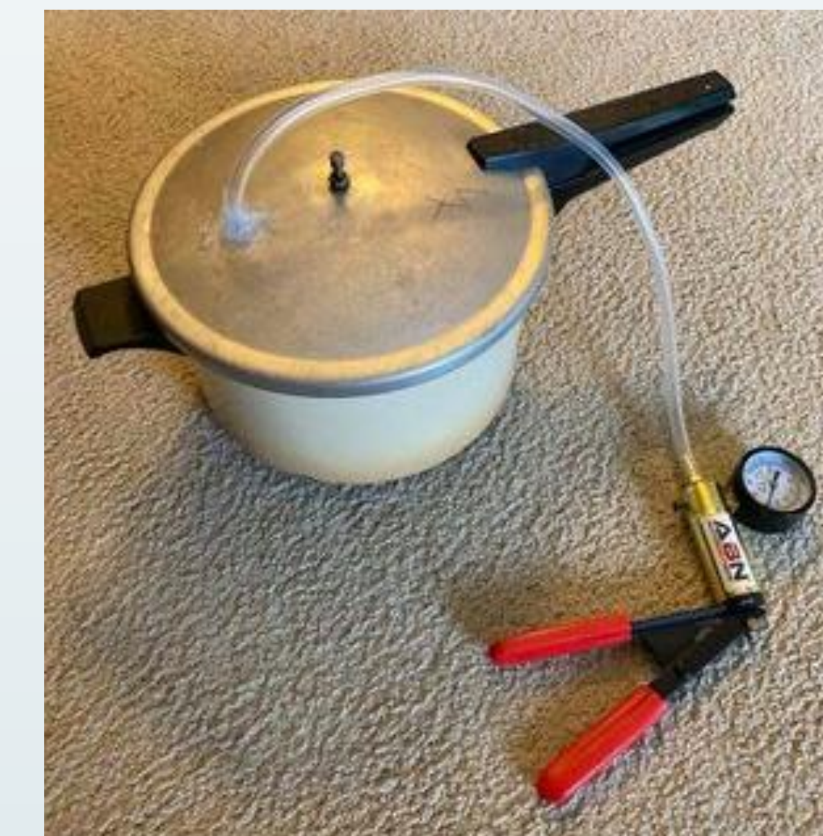
Custom-Made Vacuum Degassing System
