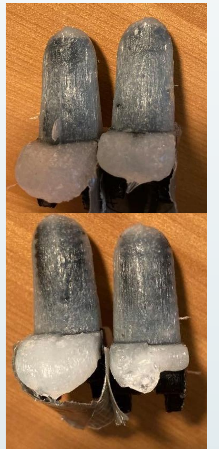
Fingertip Produced via Recommended Molding Method
