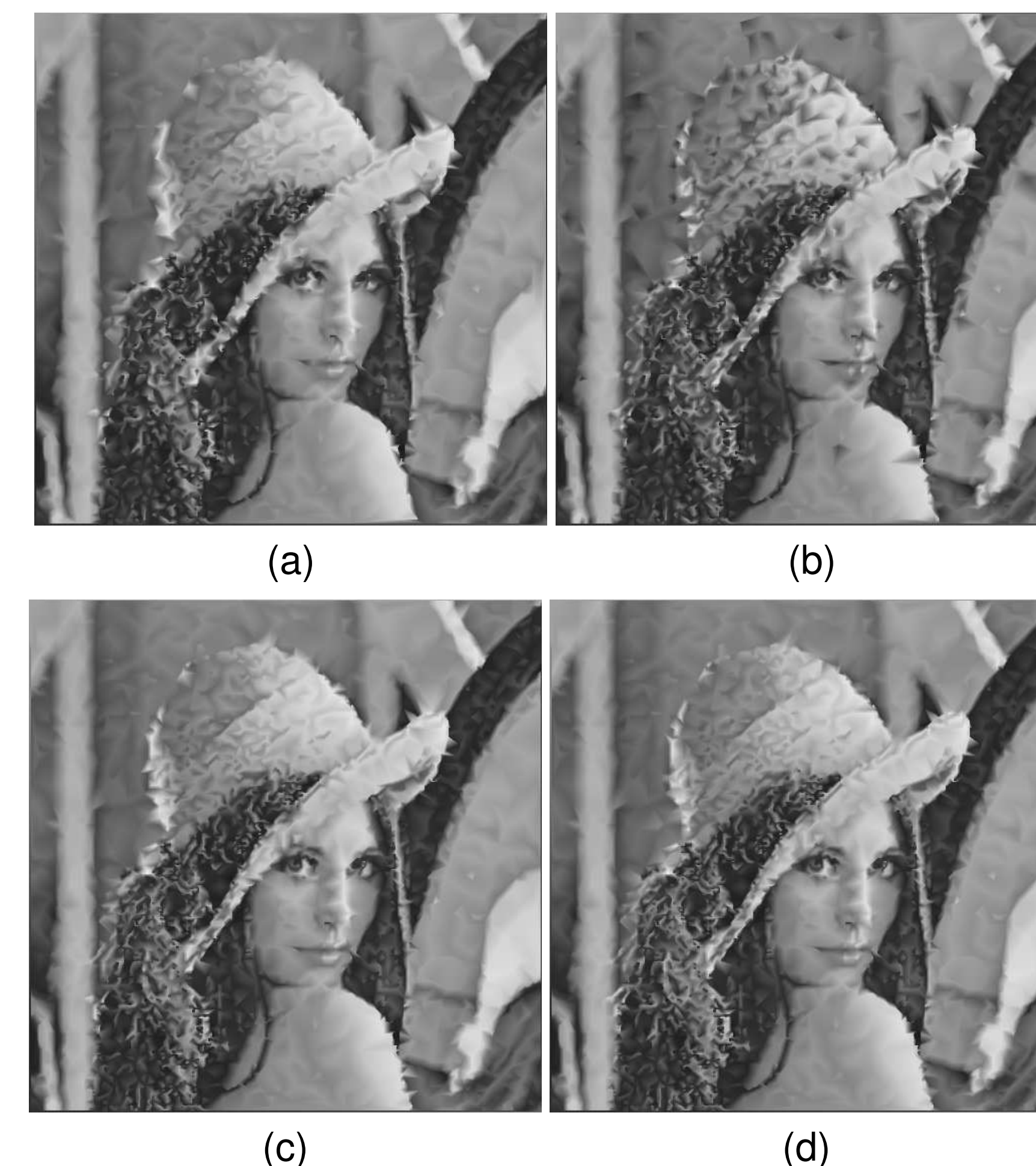
Fig. 4: Subjective image quality comparison for various sample-value ambiguity-resolution methods. Lossy reconstructions obtained at about 33:1 compression with the (a) discard (23.34 dB), (b) mean (22.11 dB), (c) nearest-neighbour (23.92 dB), and (d) median (24.37 dB) sample-value ambiguity-resolution methods.
