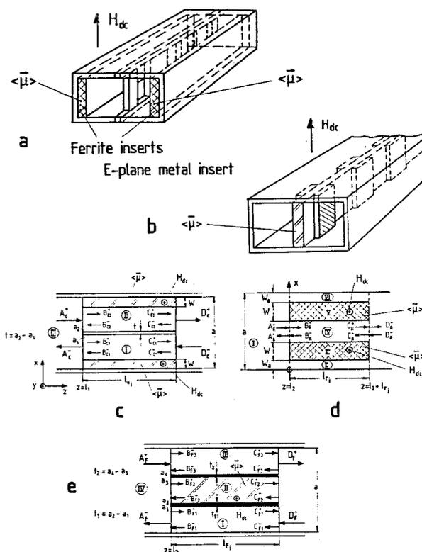
Fig. 1: Ferrite tunable millimeter wave printed circuit filters
