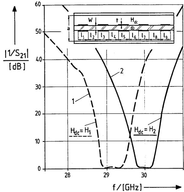
Fig. 3: Computer-optimized Ka-band magnetically tunable large-gap finline filter on a ferrite substrate
