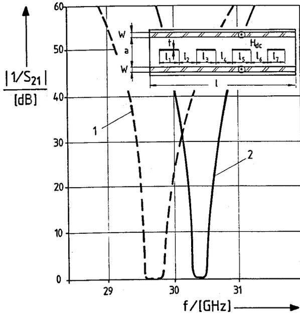
Fig. 2: Computer-optimized Ka-band magnetically tunable E-plane metal insert filter
