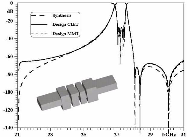
**Fig. 3** Four-pole inline  $TM_{110}$ -mode filter with three attenuation poles above the passband.
