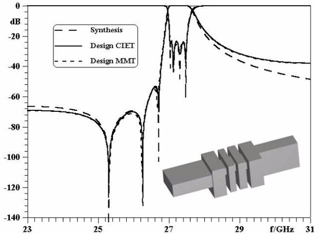
**Fig. 2** Four-pole inline  $TM_{110}$ -mode filter with three attenuation poles below the passband.
