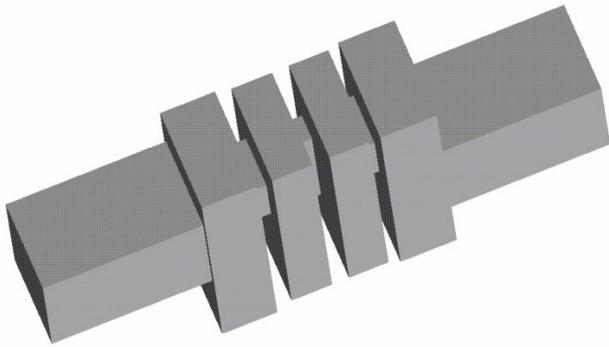
**Fig. 1** Inline waveguide filter with arbitrarily located attenuation poles.
