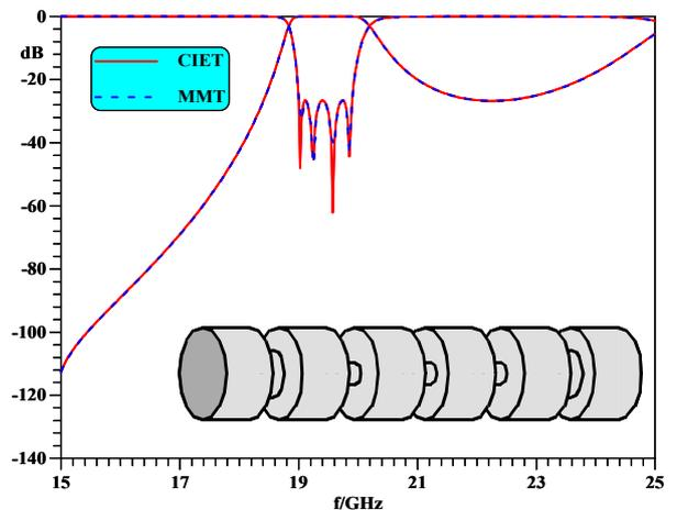
**Fig. 2** Performance of a standard four-resonator  $TE_{11}$ -mode iris filter and comparison with the MMT.
