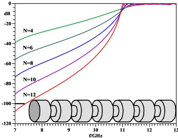
**Fig. 4** Transmission characteristics of a 'periodic' waveguide structure with  $N$  unit cells.
