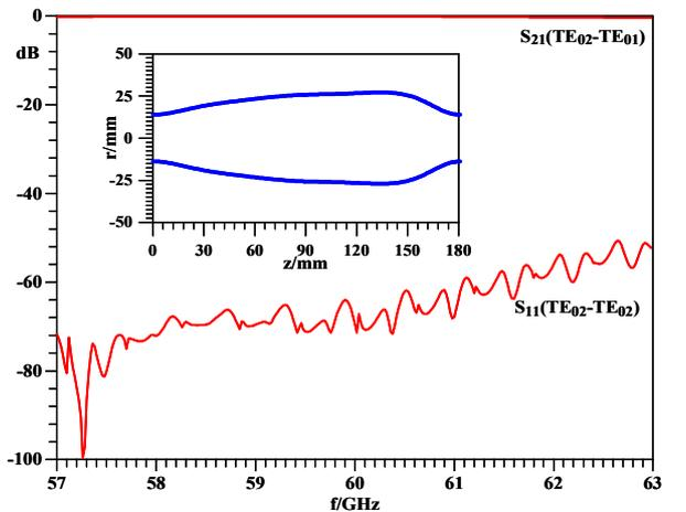
**Fig. 6** Performance of continuous-profile  $TE_{02}$ -to- $TE_{01}$  mode converter according to [2, 10].
