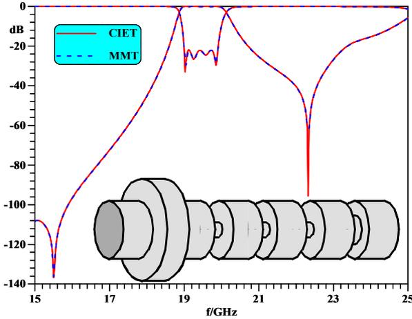
**Fig. 3** Performance of a four-resonator  $TE_{11}$ -mode filter with a single frequency-dependent inverter and comparison with the MMT.
