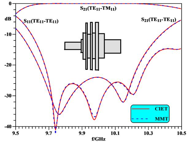
**Fig. 5** Performance of an optimized  $TE_{11}$ -to- $TM_{11}$  mode converter and comparison with MMT.
