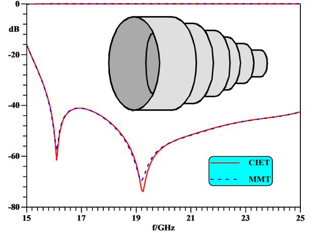
**Fig. 1** Performance of a four-section  $TE_{11}$ -mode transformer and comparison with the MMT.
