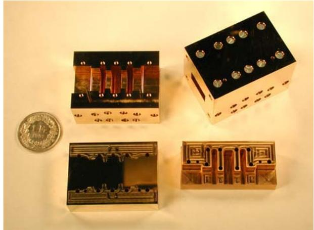
Fig. 6 Photograph of the Ku-band pseudo-highpass waveguide filter (upper right), its individually machined components and size comparison to a 1-Swiss-Franc coin.
