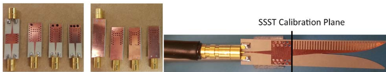
Figure 3: Custom triple short (SSST) calibration. Left: calibration standards, top plane. Middle: calibration standards, ground plane. Standards from left to right: Thru, Short1, Short2, Short3. Right: KPAF single antenna with resulting calibration plane noted.
