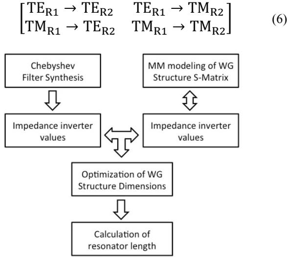
Fig. 1. Mode matching routine to obtain filter dimensions for one discontinuity.
