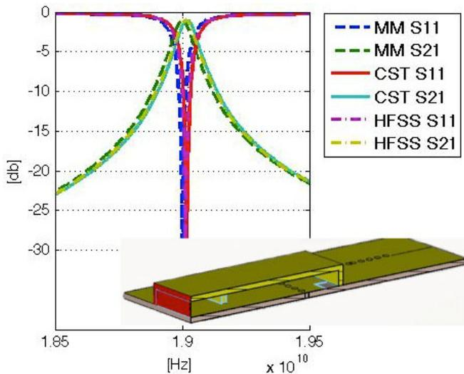
Fig. 5. Results for a single resonator SIW-SMW filter obtained with the MMT, CST, and HFSS.
