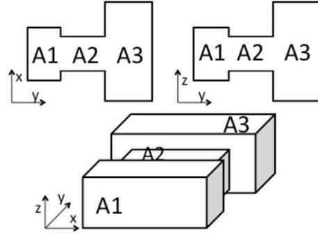
Fig. 3. Double E- and H- plane step, vector potential areas.
