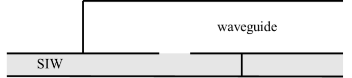
Fig. 1. Side view of the transition between SIW and substrate mounted waveguide (SMW).
