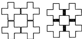
Fig. 5. Resistive-layer deposition patterns. The pattern on the right has overlaps; the pattern at left has none.
