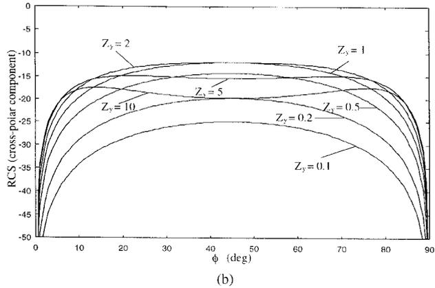
**Figure 3** (a) Monostatic copolar RCS of a square anisotropic flat plate ( $L = 76$  mm) illuminated at normal incidence ( $Z_x = 0$  and  $Z_y/\zeta = 0, 0.1, 0.2, 0.5, 1, 2, 5, 10$ ). (b) Monostatic cross-polar RCS of a square anisotropic flat plate ( $L = 76$  mm) illuminated at normal incidence ( $Z_x = 0$  and  $Z_y/\zeta = 0, 0.1, 0.2, 0.5, 1, 2, 5, 10$ )
