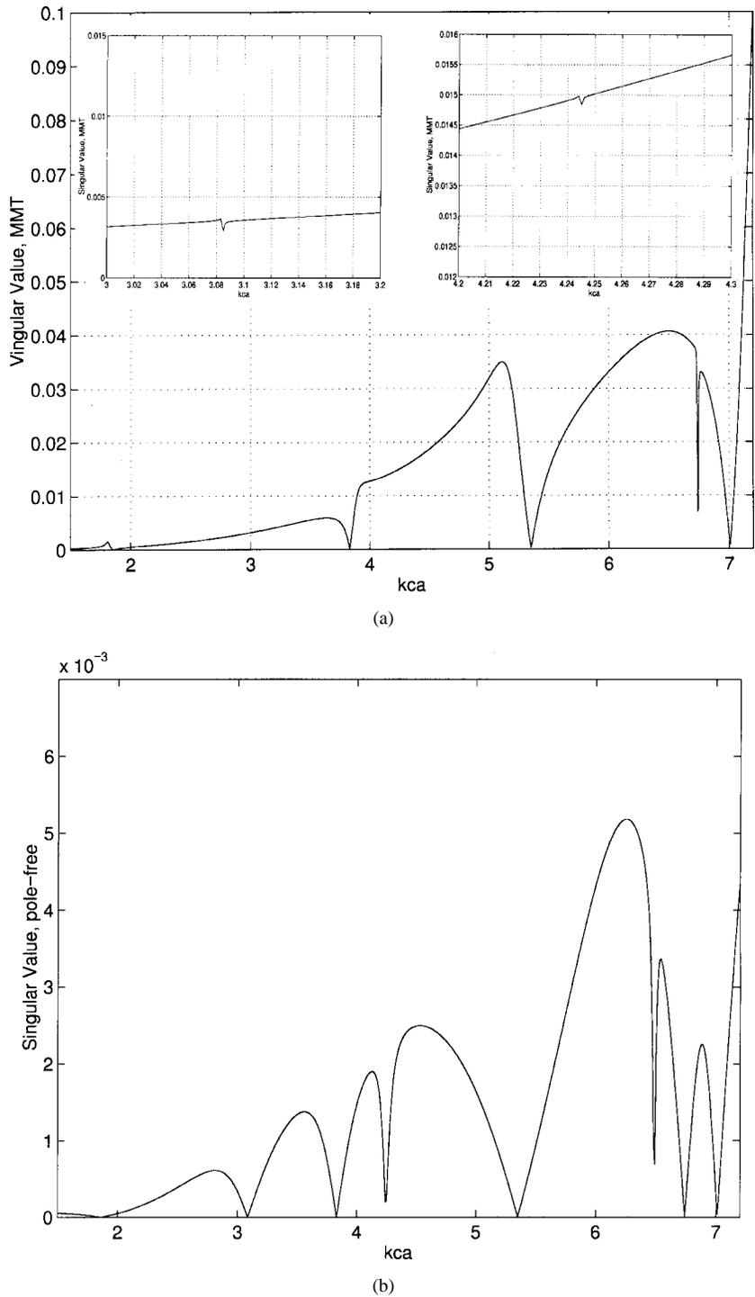
Fig. 3. Minimum singular value of  $[A(kca)]$  as a function of  $kca$  when  $h/a=0.9$ ,  $\theta=2.29^\circ$ , and  $M=N=6$ . (a) Standard MFMT and (b) pole-free MFMT.
