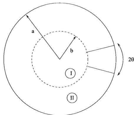
Fig. 1. Cross section of a ridged circular waveguide.
