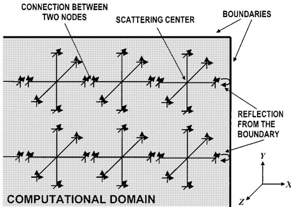
Fig. 1. Discretization mesh of the FDTLM nodes.
