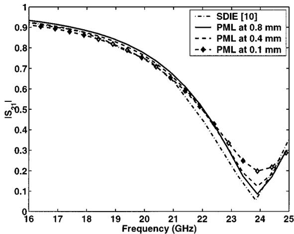
Fig. 8. Transmission coefficient of the CPW resonator with L-shaped stubs. PML absorbers are used as the absorbing boundaries.
