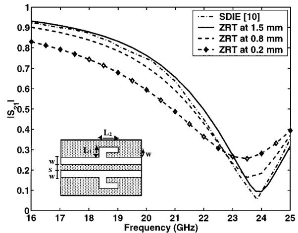
Fig. 6. Transmission coefficient of the CPW resonator with L-shaped series stubs.  $w = 0.225$  mm,  $s = 0.45$  mm,  $L_1 = 0.45$  mm, and  $L_2 = 1.125$  mm. Substrate thickness  $h = 0.635$  mm and  $\epsilon_r = 9.9$ .
