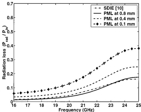
Fig. 9. Radiation loss  $1 - |S_{11}|^2 - |S_{21}|^2$  of the CPW resonator with L-shaped series stubs obtained for various distances between the PML absorber and resonator structure.
