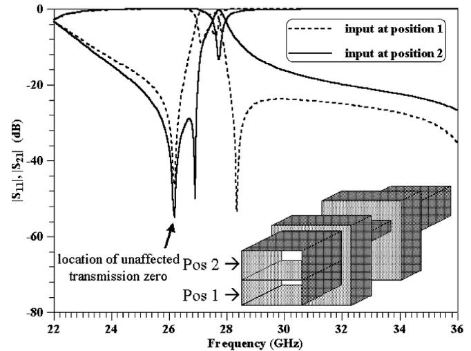
Fig. 5. Effect of moving the input coupling aperture of two cascaded singlets. One transmission zero remains unaffected.
