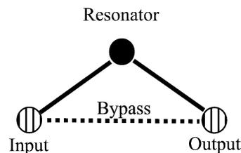
Fig. 1. Coupling and routing scheme of a singlet: one resonator with one transmission zero.
