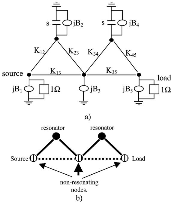
Fig. 2. Nonresonating node model (NRNM) of two cascaded singlets. (a) Equivalent low-pass network and (b) coupling and routing scheme.
