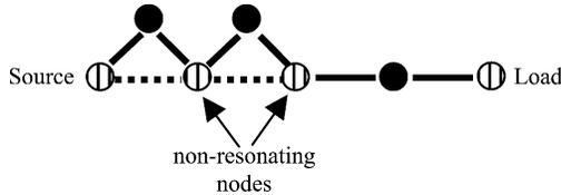
Fig. 3. Nonresonating node model (NRNM) of a third-order filter with two cascaded singlets and one additional resonator. Dark disks: resonators; patterned disks: nonresonating nodes.
