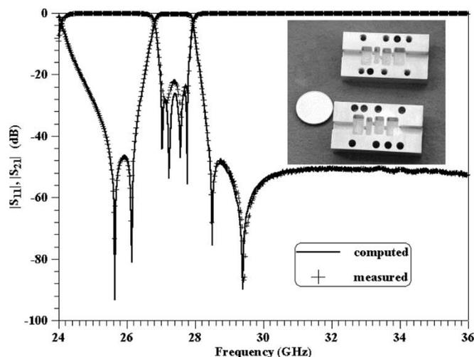
Fig. 7. Measured (+) and simulated (–) response of a fourth-order elliptic filter implemented by cascading four singlets in  $TM_{110}$ -mode rectangular cavities.
