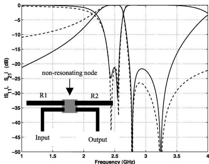
Fig. 6. Reflection and transmission coefficients of two cascaded singlets in two-layer microstrip technology. Solid lines: full-wave (IE3D), dashed lines: coupling matrix.
