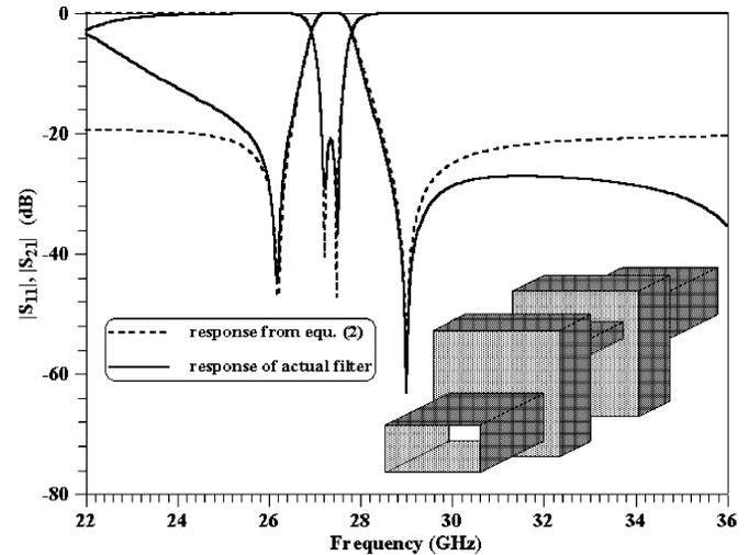
Fig. 4. Transmission and reflection coefficient of two cascaded singlets yielding a symmetric response. Solid lines: full wave (CIET), dashed lines: coupling matrix (2).
