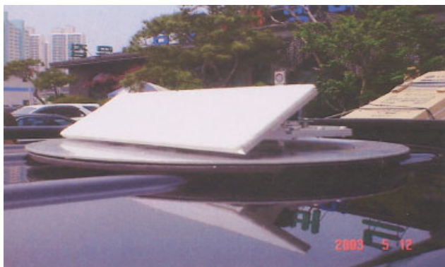
Figure 9 Photograph of the proposed array antenna mounted on the rooftop of the vehicle. [Color figure can be viewed in the online issue, which is available at www.interscience.wiley.com .]
