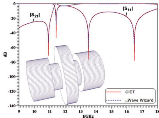
Fig. 5. Performance of an extended  $TM_{110}$ -mode singlet incorporating resonances of irises and that of the  $TE_{111}$  mode.
