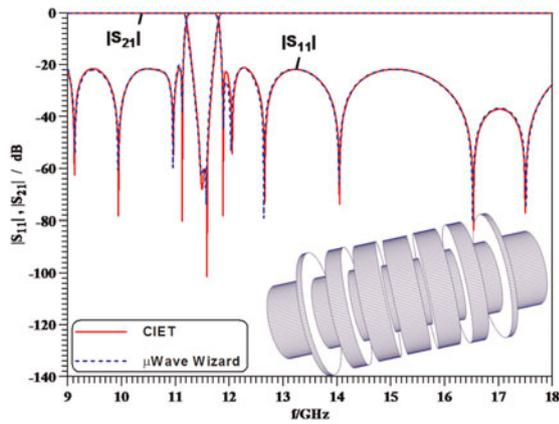
Fig. 7. Performance of a bandstop filter with seven  $TM_{110}$ -mode resonators; dimensions cf. Table 1.
