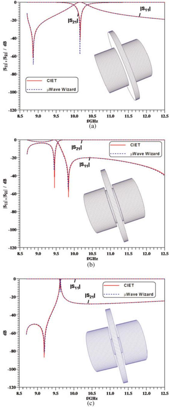
Fig. 2. Performance of a  $TM_{110}$ -mode cavity coupled to standard circular WC 80 waveguides: (a) direct coupling, (b) through large irises, and (c) through small irises.
