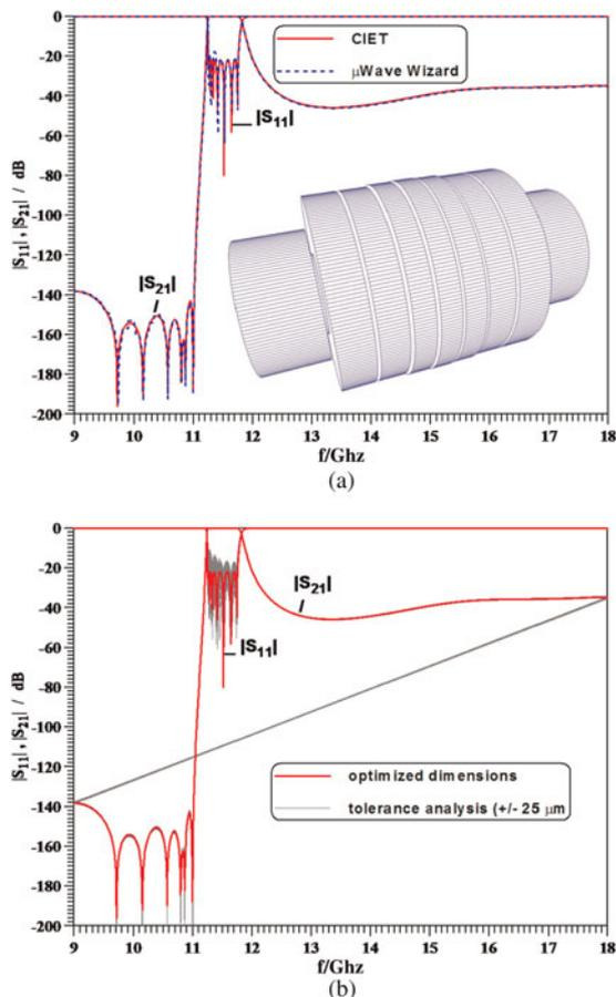
Fig. 4. Performance of a seven-resonator  $TM_{11}$ -mode filter (Table 1) for comparison with Fig. 1: (a) S parameters and (b) tolerance analysis.
