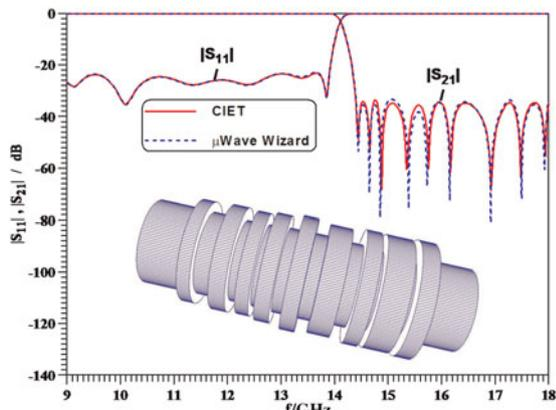
Fig. 8. Performance of a lowpass filter with nine  $TM_{110}$ -mode resonators; dimensions cf. Table 1.
