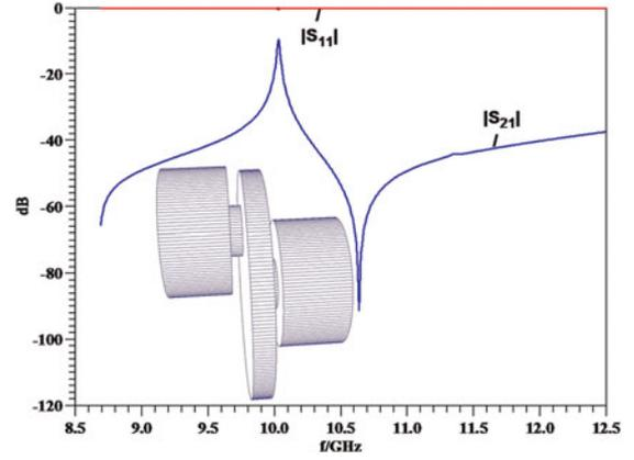
Fig. 3.  $\mu$ Wave Wizard computation of an offset-connected  $TM_{010}$ -mode cavity with the transmission zero to the right of the resonance.
