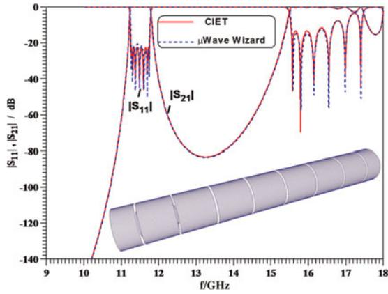
Fig. 1. Performance of a seven-resonator regular circular waveguide iris filter designed for 500 MHz bandwidth at 11.5 GHz (cf. Table 1).
