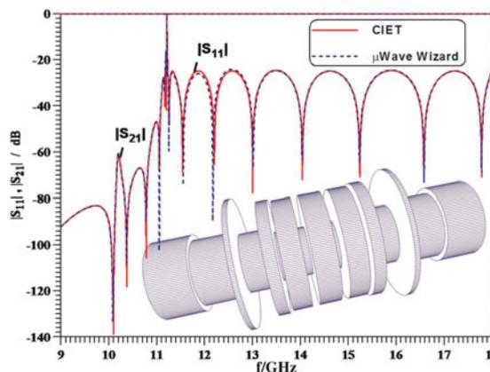
Fig. 6. Performance of a quasi-highpass filter (Table 1) with seven  $TM_{110}$ -mode resonators and additional resonances according to Fig. 5.
