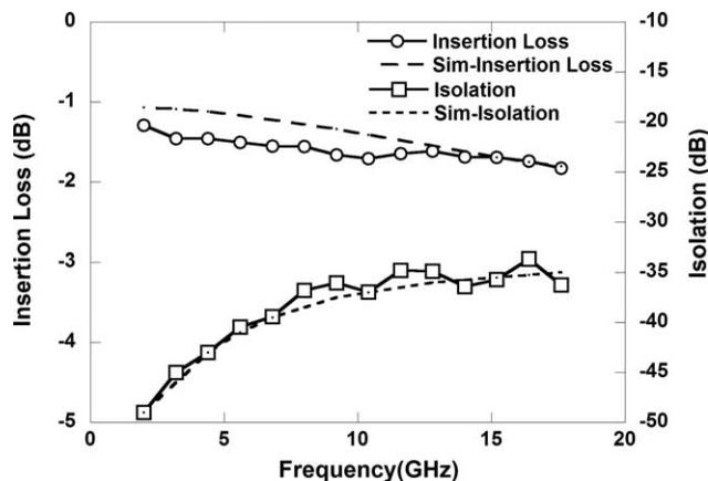
**Figure 12** Simulated and measured results of insertion loss and isolation of PIN diode SPDT switch
