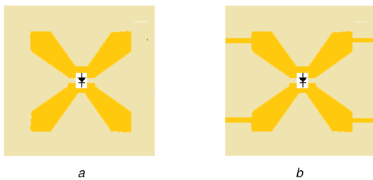
Fig. 4 Four-arms star geometry with PIN diode (a) PIN diode inserted, (b) Bias lines added
