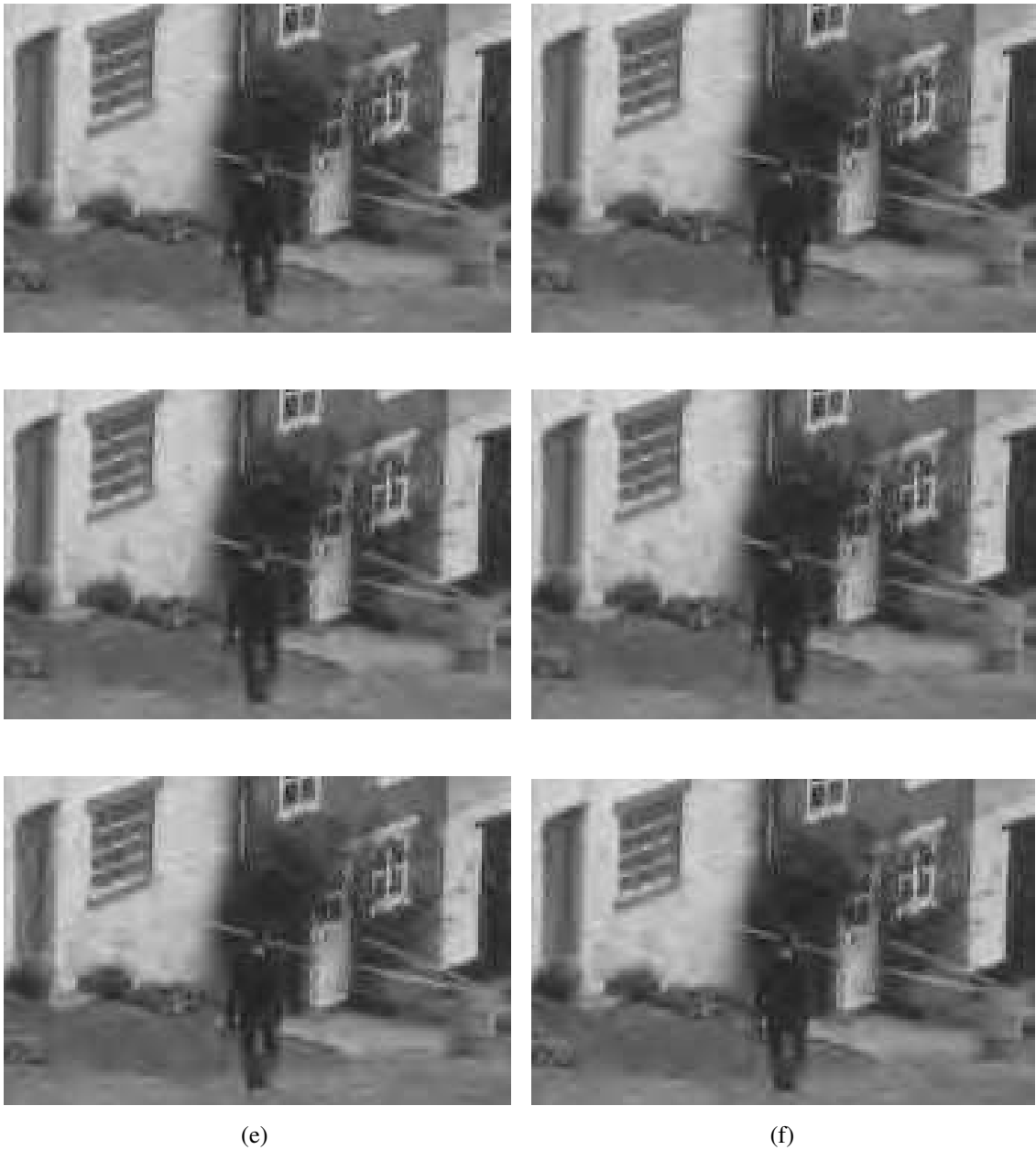
Figure 3.10: Parts of the lossy reconstructions obtained after coding the gold image at a compression ratio of 32:1 using the (a) 9/7, (b) 9/11, (c) 13/11, (d) 17/11, (e) 13/15, and (f) 9/7-J filter banks.
