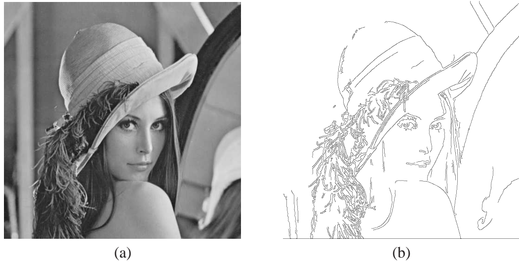
Figure 2.12: Example of edge detection. (a) The original image, and (b) the edge map produced by the edge detector.
