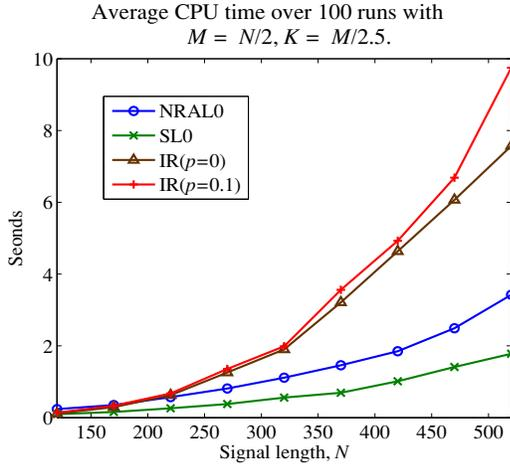
Fig. 2. Average CPU time required by the IR, SL0, and NRALO algorithms over 100 runs.
