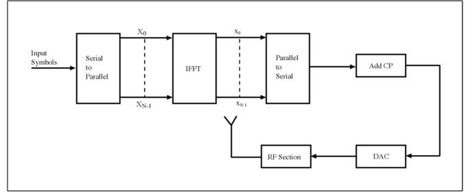
Figure 1: The basic structure of an OFDM transmitter.
