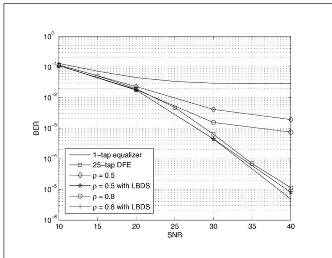
Figure 7: BER performance of the two-dimensional bounded constraint relaxation method with various thresholds and  $f_d T_s = 0.1$  in a 16-QAM OFDM system.
