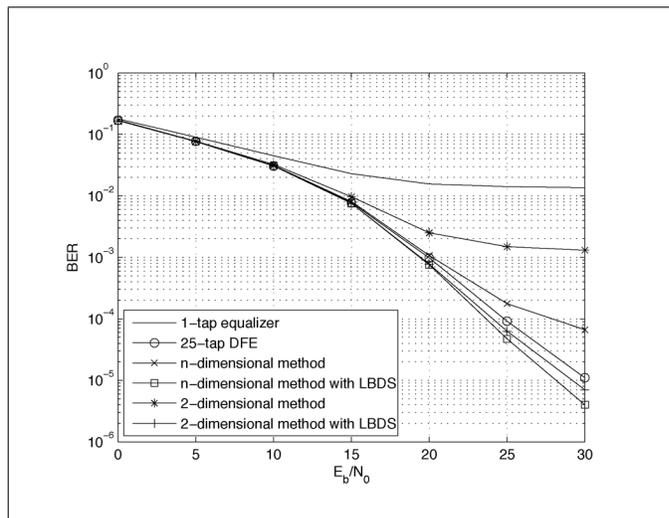
Figure 5: BER performance of the quadratic constraint relaxation method with  $f_d T_s = 0.1$  in a 4-QAM OFDM system.
