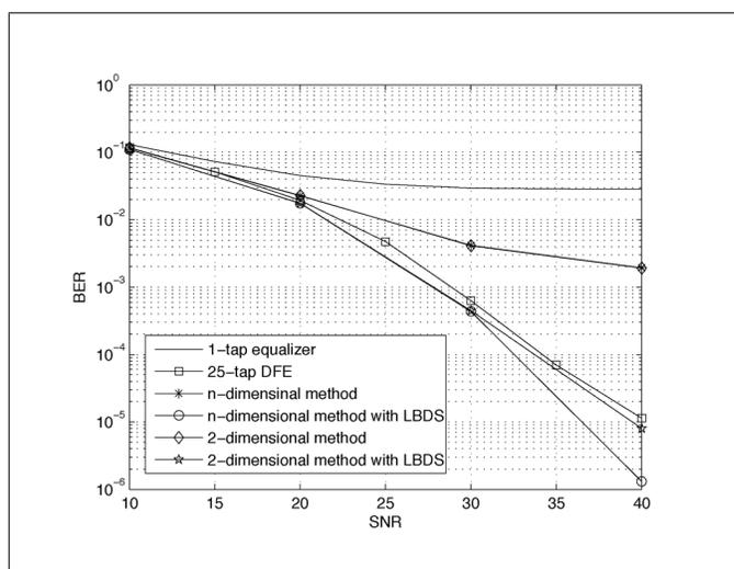
Figure 6: BER performance of the bounded constraint relaxation method with  $\rho = 0.5$  and  $f_d T_s = 0.1$  in a 16-QAM OFDM system.
