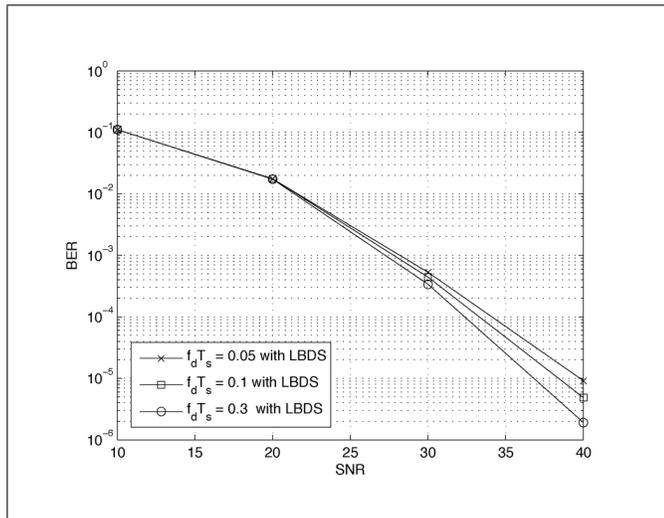
**Figure 10:** BER performance of the two-dimensional bounded constraint relaxation method with various Doppler spreads in a 16-QAM OFDM system.
