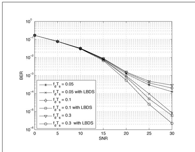
Figure 9: BER performance of the two-dimensional bounded constraint relaxation method with various Doppler spreads in a 4-QAM OFDM system.
