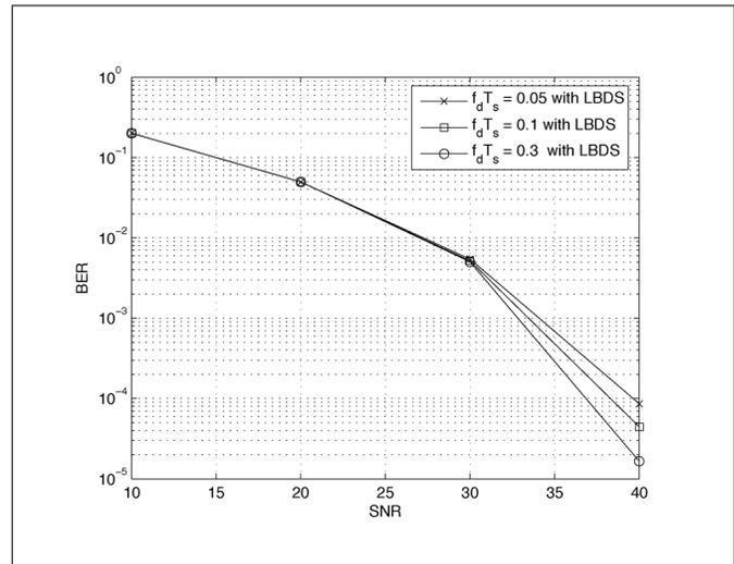
**Figure 11:** BER performance of the two-dimensional bounded constraint relaxation method with various Doppler spreads in a 64-QAM OFDM system.
