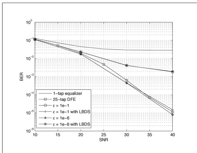
Figure 8: BER performance of the bounded constraint relaxation method with  $f_d T_s = 0.1$  for various values of  $\epsilon$  in a 16-QAM OFDM system.
