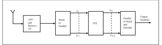
Figure 2: The basic structure of an OFDM receiver.
