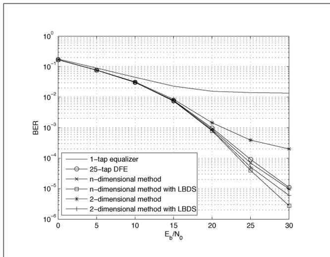
Figure 4: BER performance of the bounded constraint relaxation method with  $f_d T_s = 0.1$  in a 4-QAM OFDM system.
