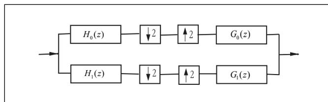
Figure 1: A two-channel CQ filter bank.
