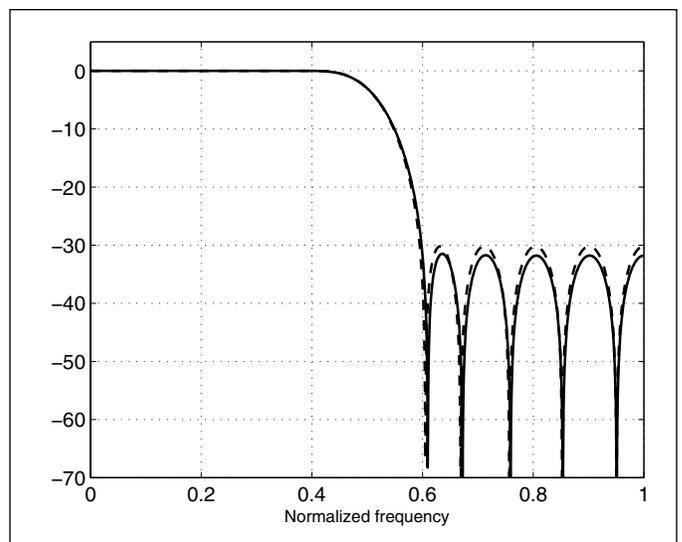
Figure 9: Magnitude responses of minimax  $H_0(z)$  with  $N = 20$  of the global design (solid line) versus that of  $H_0(z)$  in [14] (dashed line).
