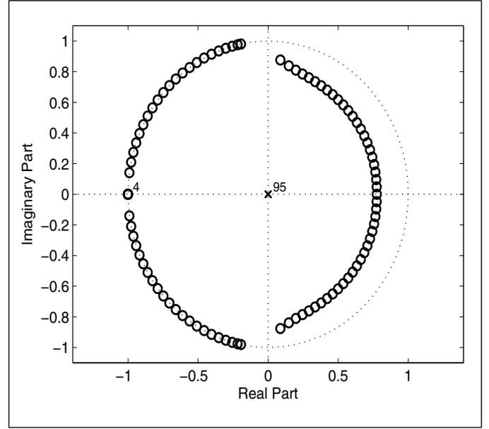
Figure 5: Zero-pole plot of LS  $H_0(z)$  with  $N=96$ ,  $L=3$  and  $\omega_a=0.56\pi$ .
