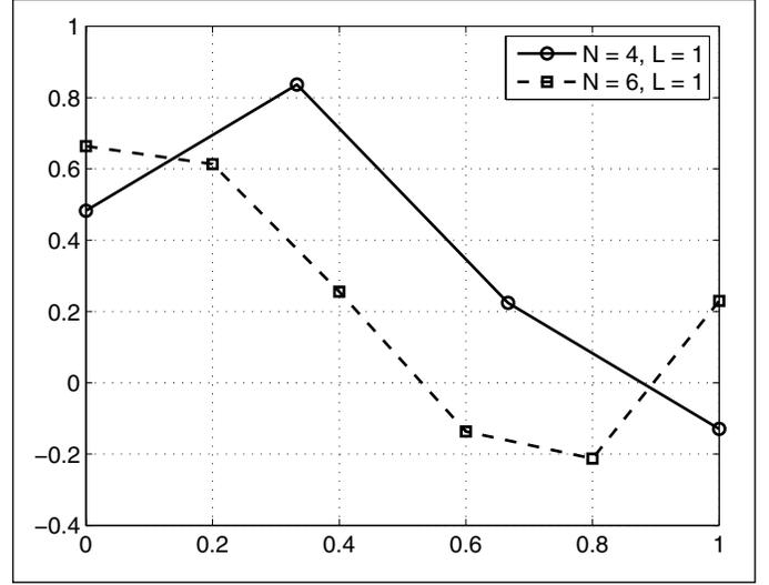
Figure 6: Pattern of minimax impulse responses with different length  $N$ .
