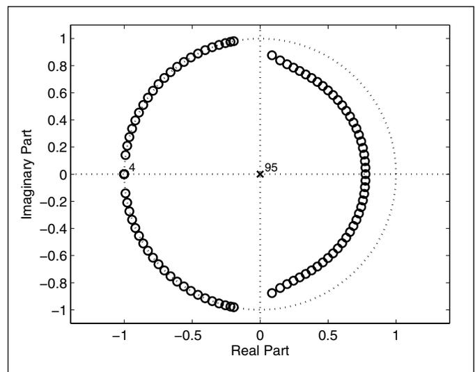
Figure 8: Zero-pole plot of minimax  $H_0(z)$  with  $N = 96$ ,  $L = 3$  and  $\omega_a = 0.56\pi$ .
