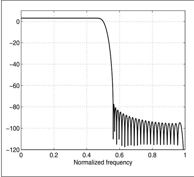
Figure 4: Magnitude response of LS  $H_0(z)$  with  $N=96$ ,  $L=3$  and  $\omega_a=0.56\pi$ .
