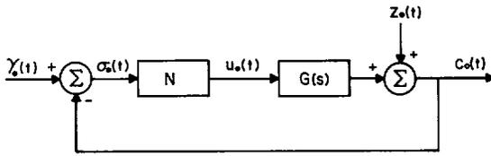
Fig. 1. Nonlinear feedback system.
