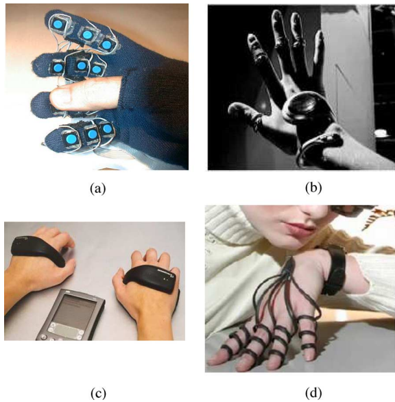
Fig. 7. Gloves for portable/wearable computers. (a) Thumbcode. Image courtesy V. Pratt. (b) Scurry [134]. © 2005 IEEE. (c) Senseboard. Image courtesy Senseboard Technologies. (d) Design study of KITTY glove. Image courtesy C. Mehring.
