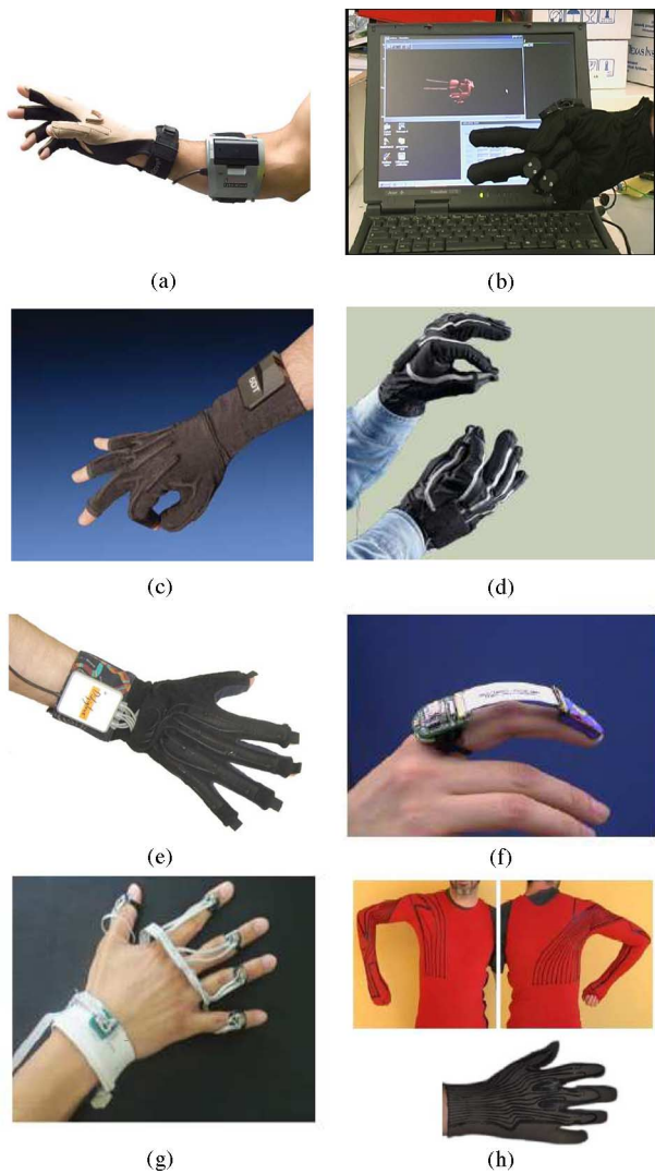
Fig. 2. Glove systems. (a) CyberGlove II. Reproduced by permission of Immersion Corporation. Copyright © 2008 Immersion Corporation. All rights reserved. (b) Humanglove. Image courtesy Humanware. (c) 5DT Data Glove. Image courtesy www.5dt.com. (d) Pinch Glove. Image courtesy Fakespace Systems. (e) Didjiglove. Image courtesy John Timlin, Didjiglove Pty. Ltd., Melbourne, Australia. (f) Fingernail Sensor [186]. Image courtesy H. H. Asada. (g) AceleGlove [15]. Copyright © ACM. Reprinted by permission. (h) Upper limb garment prototype [187] and sensing glove [188] by Pisa University: sensors are directly integrated in Lycra fabrics by using conductive elastometers sensors. © 2006 IEEE and © 2005 IEEE.
