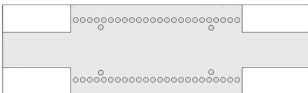
**Fig. 11** Top view of the designed SIW filter with microstrip ports
