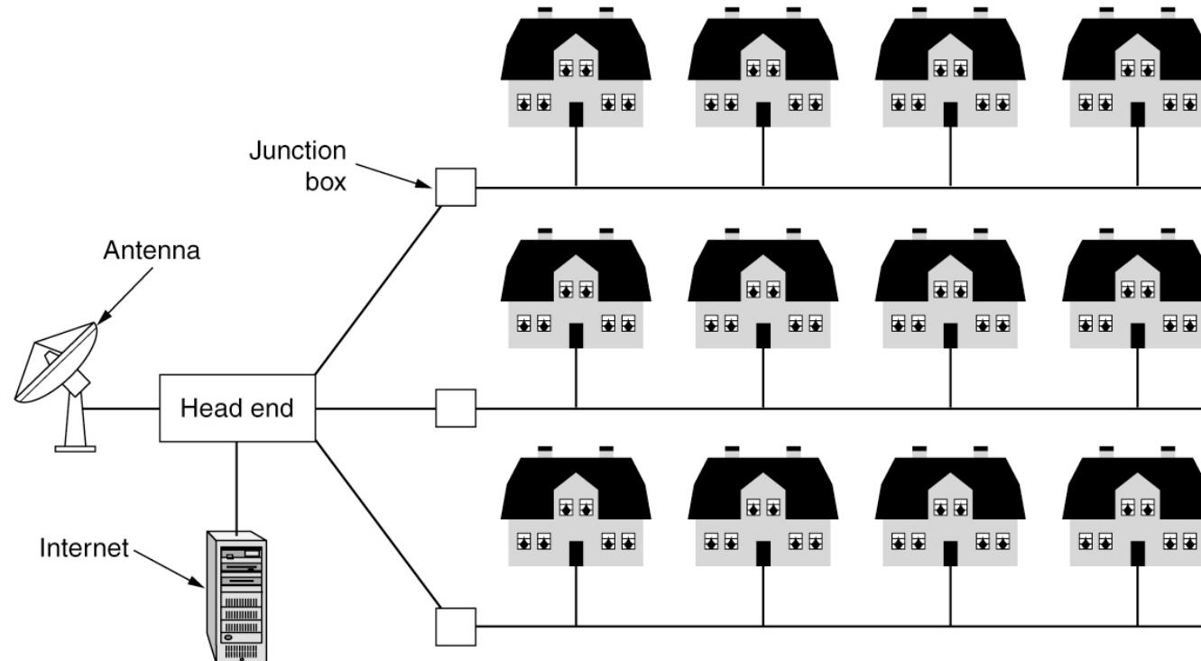
A Metropolitan Area Network (MAN) where both television signals and the Internet are fed into the cable head-end (or cable modem termination system) for subsequent distribution to homes.
