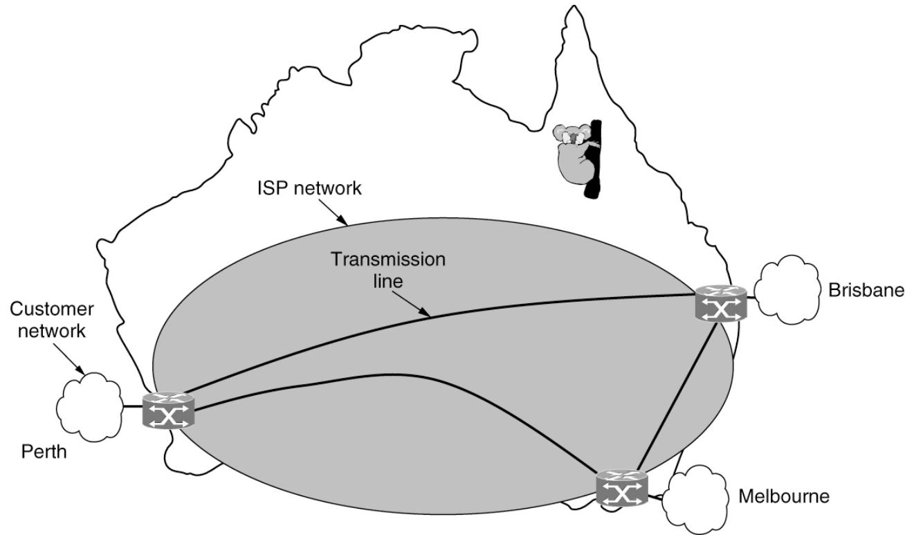
A wide area network with hosts in Perth, Brisbane, and Melbourne connected via an ISP.
