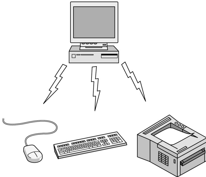
Personal Area Networks (PANs) let devices communicate over the range of a person. Bluetooth is a short-range wireless technology used to connect components without wires.
