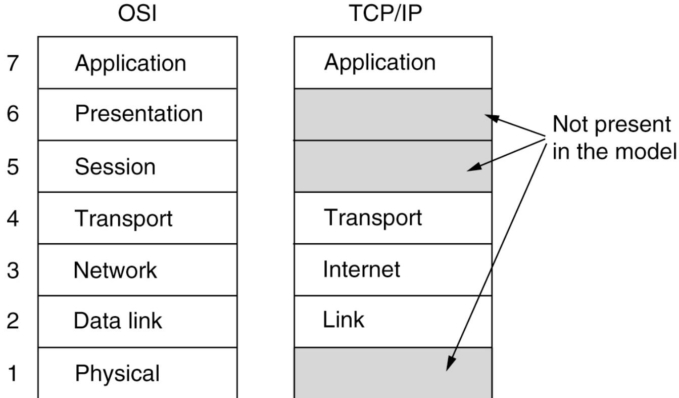
The TCP/IP layers loosely align with the OSI model.
