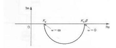
Polar plot of a lag compensator  $K_{\alpha}\beta(j\omega T+1)/(j\omega\beta T+1)$
