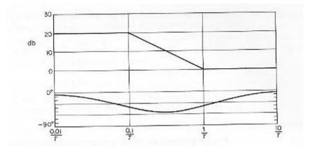
Bode diagram of a lag compensator with  $K_c=1$ ,  $\beta = 10$
