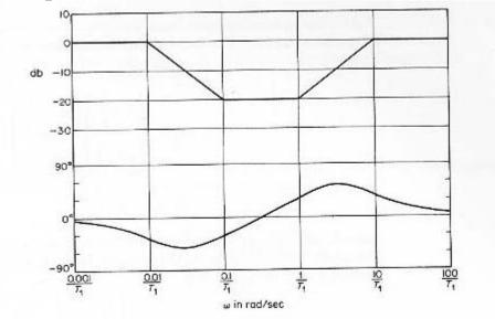
Bode diagram of a lag-lead compensator given by
