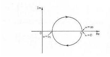
Polar plot of a lag-lead compensator given by
