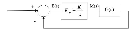
$$\frac{M(s)}{E(s)} = K_p + \frac{K_i}{s} = \frac{K_p s + K_i}{s} \qquad m(t) = K_p e(t) + \int K_i e(t) dt$$
